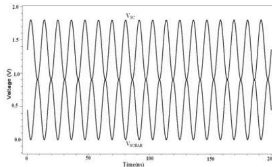
Fig 1b. Split level Sinusoidal power clock
