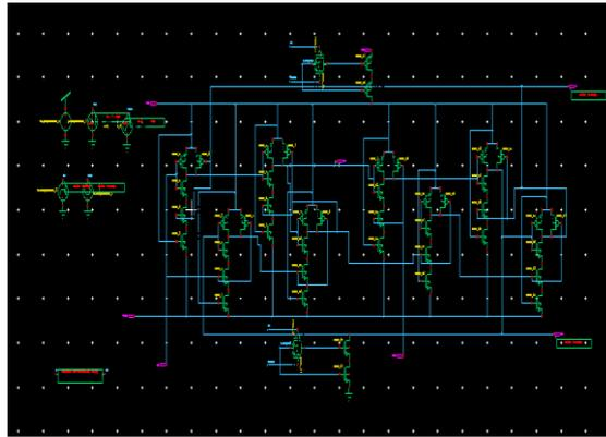
Fig 1.6 Schematic Diagram of Frequency divider using stacking technique
