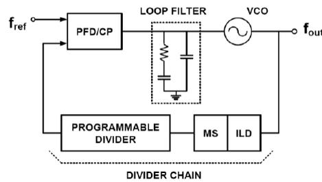
Fig 1.4 Millimetre-wave PLL frequency synthesizer architecture.
