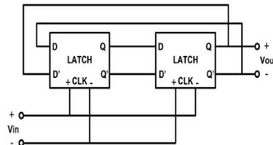
Fig 1.3 Master-Slave frequency divider block diagram.
