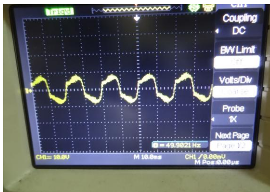
Fig.17. Experimental Waveform for Generator side voltage, CH2=10V/div
