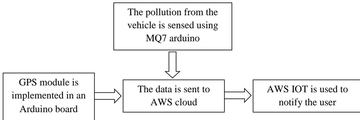
**Fig 1. System Architecture**
